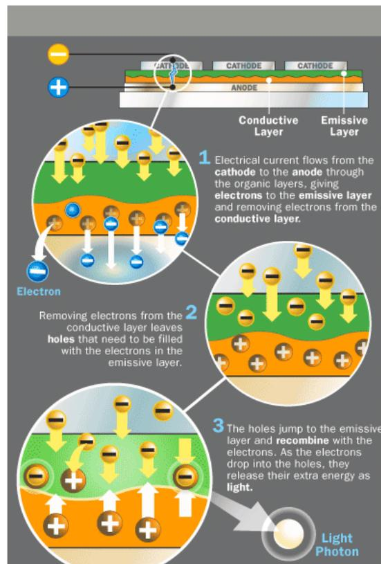
Fig.6- Working Layout of OLED [5]
