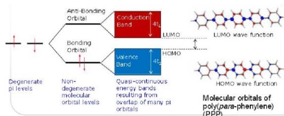
**Fig 3** Bondings in OLED structure
