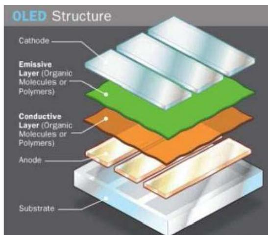
**Fig.4-** Layers of OLED [5]
